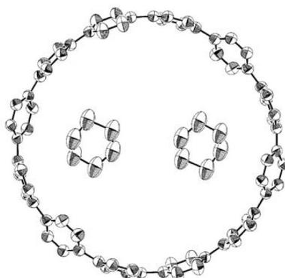
This x-ray structure is closer to *D*<sub>3d</sub> form which has higher energy (by 3.7 kcal/mol) than most stable *D*<sub>6d</sub> form, indicated by DFT calculation.
