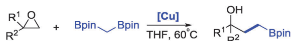
Scheme 1 Previous studies on transition metal catalyzed Suzuki Miyaura cross-coupling reaction of epoxides.
